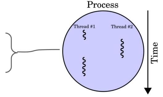
A process with two threads of execution, running on a single processor [wiki]
