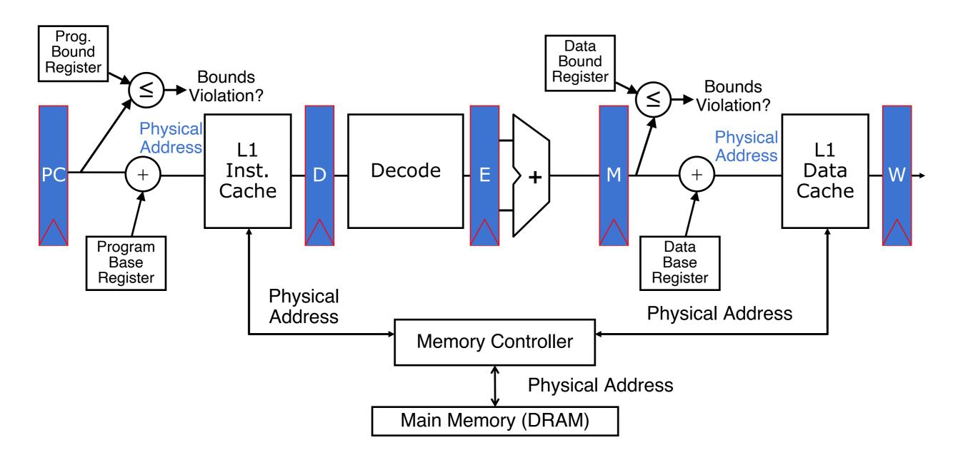
Can fold addition of base register into (register+immediate) address calculation using an adder
