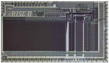
RISC-II (1983) contains 40,760 transistors, was fabbed in 3 µm NMOS, ran at 3 MHz, and the size is 60 mm<sup>2</sup>.
