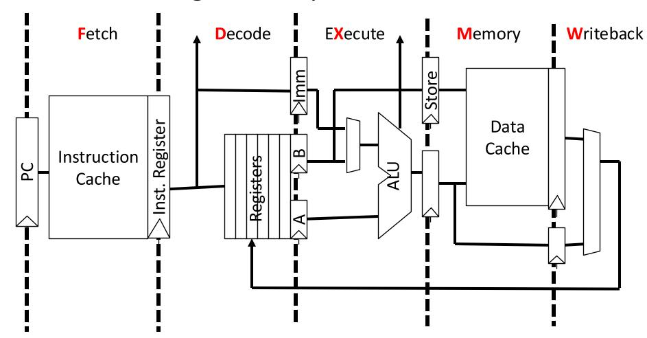
This version designed for regfiles/memories with synchronous reads and writes.
