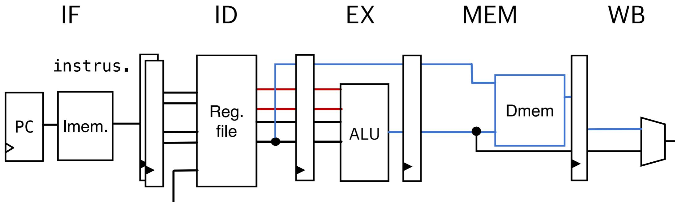
Hardware has to be adapted to avoid structural hazards
