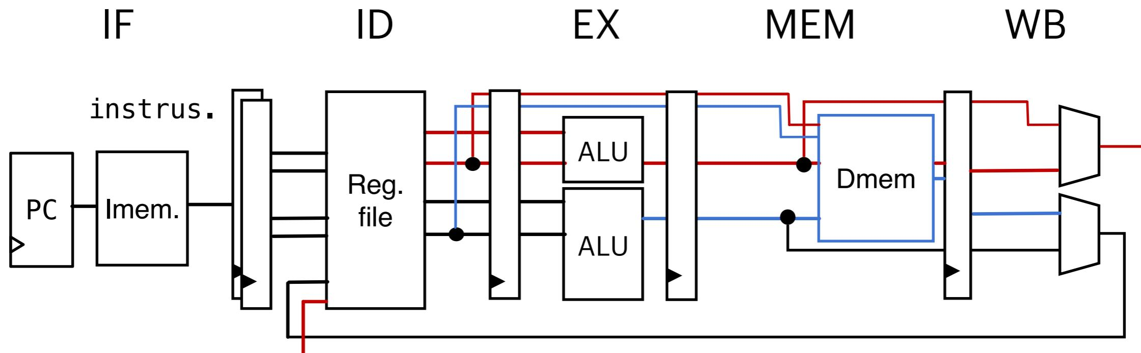
Hardware has to be adapted to avoid structural hazards
