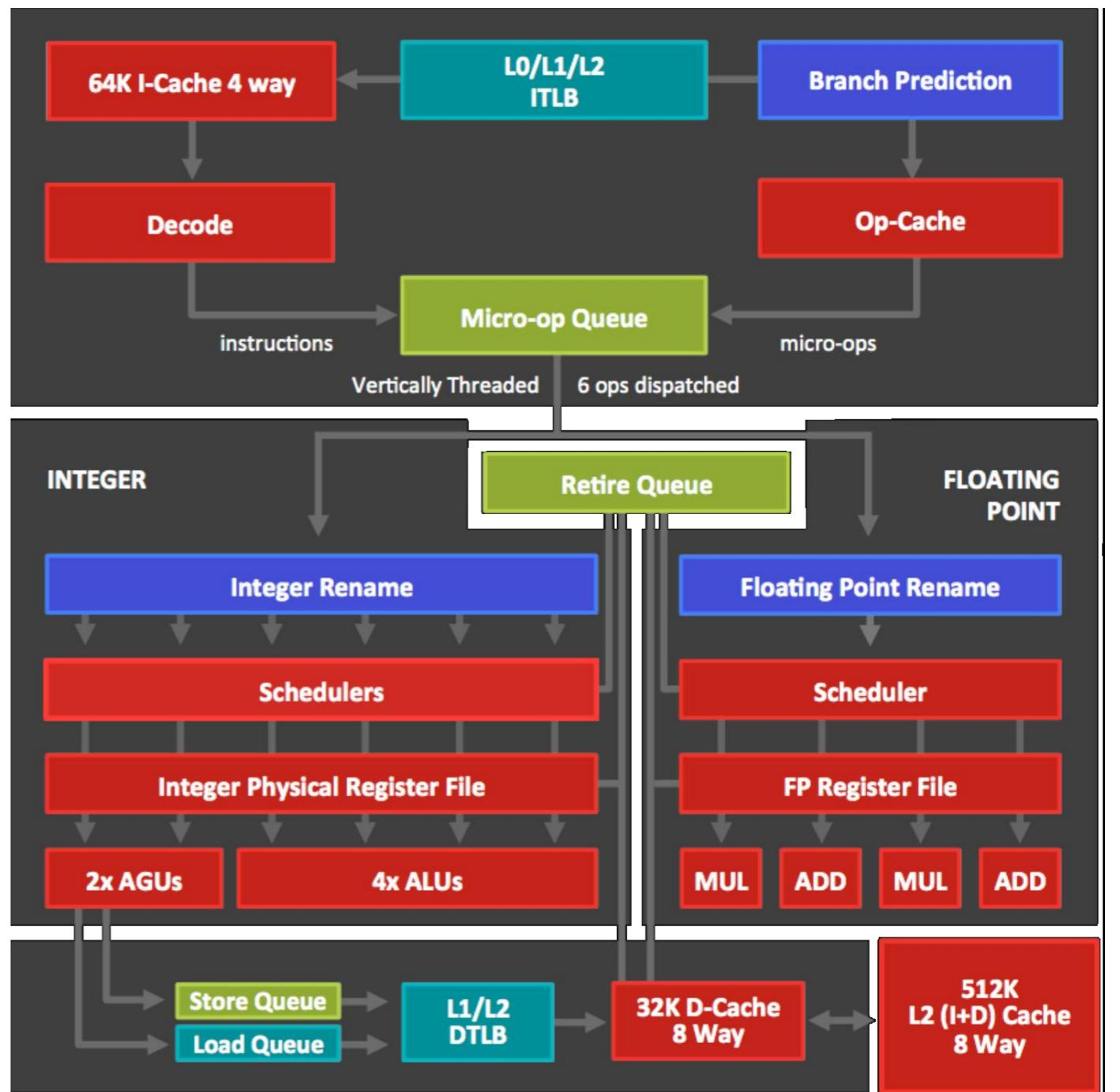
AMD CPU (Zen architecture) that supports simultaneous multithreading
